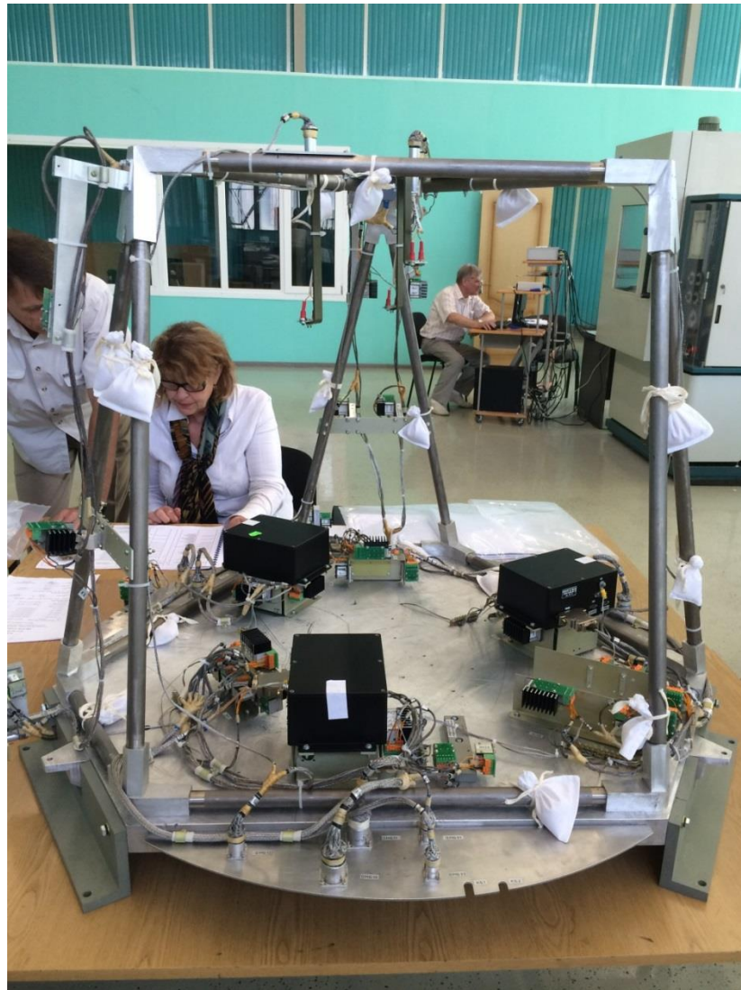
Рис.3. Electrical model of WUVS instrument.
