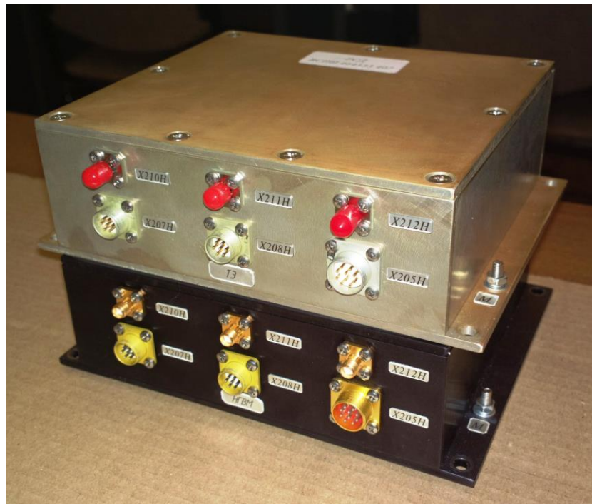
Fig.2. General view of the RSD receiver. Thermal equivalent (top). Full-scale prototype (bottom).
